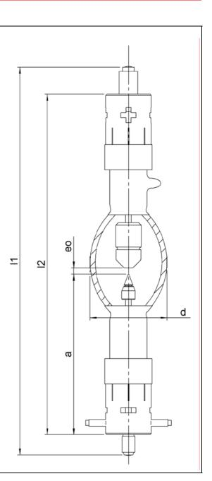
\*) w = luminance half width value; h = height of luminous area (corresponds to electrode gap, hot)
